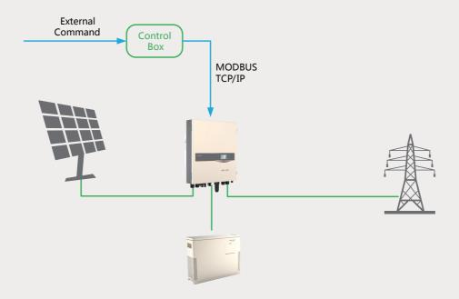
With the MODBUS TCP/IP protocol, the SH5K hybrid inverter can be manually configured via Control Box to shutdown, startup, active power derating, reactive power regulation, or charge/discharge power control etc..
